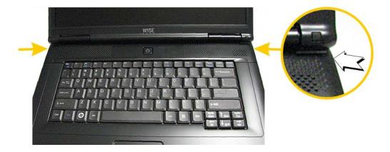
5. Using the plastic alignment tool carefully lift up the keyboard (start lifting at the arrow shown in Figure 7), and then lay keyboard facedown to expose the flash and memory modules.
